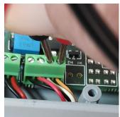
Put a piece of your label material in the sensor. Make sure it rests on the bottom of the sensor. Around 2,0 Volts should be measured on the label and around 0,3 to 0,5 Volts on the backing paper of the label.
